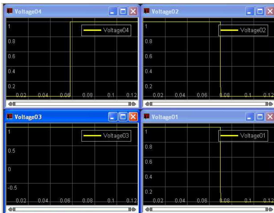
Figure 3.14 Control Signal from TBA, SA2, SA1 and SBA for Fault 1 (starting with upper left corner and reading column wise)
